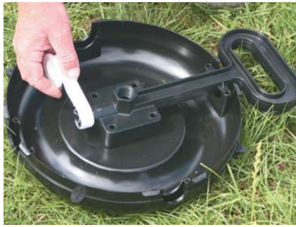
Thread tape the end of the handle.
