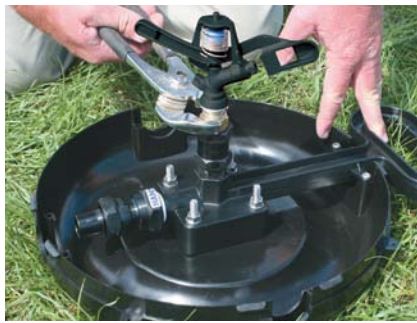
Screw the 20mm sprinkler into the socket.
