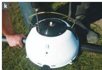
Locate Pop-up Pod Cover on top of Irripod Top Cover and ensuring the cutouts in the Pop-up Cover locate inline with the Pipe direction, fasten with screws.
