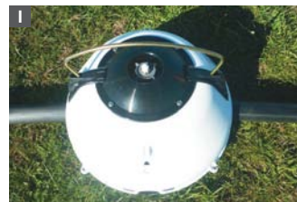
Flush the irrigation line prior to fitting the pipeline Tow Eye to remove any drilling debris left in the pipe.
