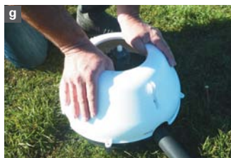
Locate body on skid base and push firmly down to engage grip lugs.
