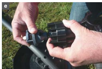
Tip the Pop-up TST until Mini Reg or Riser protrude, hold with finger and screw on Nelson R2000WF. Note all threads should be hand tight, do not use a tool for tightening.
