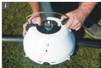
Fix wire clip into opposing holes on body sides.
