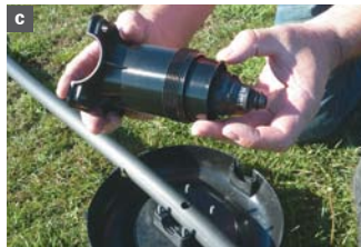
Screw either Nelson Mini Reg or Irripod ACME Male/Female High Riser onto ACME thread in base of Pop-up Piston and then place into Pop-up Tapping Saddle Top
